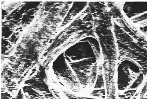
Laboratory made paper from Pinus radiata kraft (chemical) pulp
